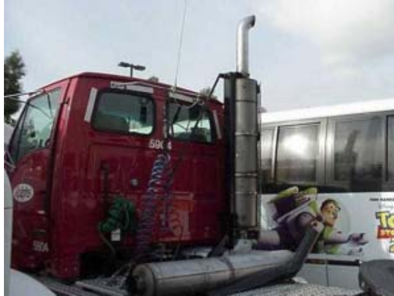
Source: Manufacturers of Emissions Controls Association shows a truck retrofitted with a diesel particulate filter.
